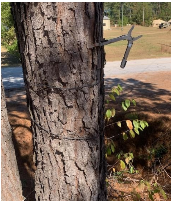
A field-expedient antenna is created by using copper wire wrapped around a knife stuck into a pine tree with an RF cable wrapped around the tree trunk three times. (Photo by Sgt. 1st Class Sandy Baron, U.S. Army Signal School)
