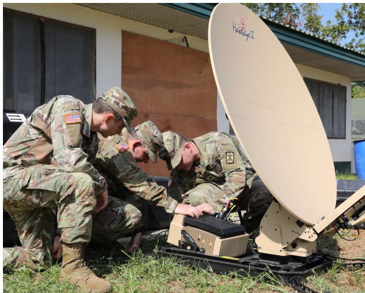
Soldiers with 307th Expeditionary Signal Battalion-Enhanced install set up their Scalable Network Node during Salaknib 2023. (Photo by Capt. Stacey Lasay, 2nd Infantry Brigade Combat Team Public Affairs Office)
